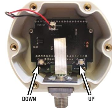
With the gauge off, press and hold the DOWN calibration button, and also press the front button.
